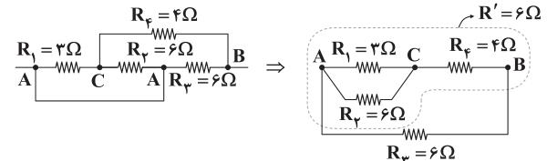
$$R'' = \frac{R' \times R_3}{R' + R_3} = \frac{6 \times 6}{6+6} = 3\Omega$$
