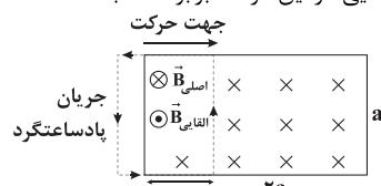
$$I_1 = \frac{Bv\ell}{R} = \frac{^{\circ}/_4 \times 10 \times ^{\circ}/_1}{^{\circ}/_1} = ^{\circ}/_0 4 A = 40 \text{ mA}$$
